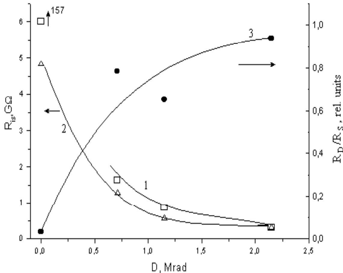
*Interstrip resistance for the detectors without (1) and with (2)  $Si_3N_4$ . Interstrip resistances ratio for the detectors with double-layer and single-layer insulation (3).*
