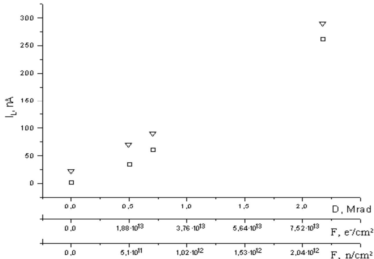
*Leakage currents variation for microstrip detectors with ( $\triangledown$ ) and without  $\text{Si}_3\text{N}_4$  ( $\square$ )*
