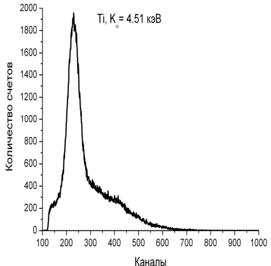
**Measurement of the radiation energy
