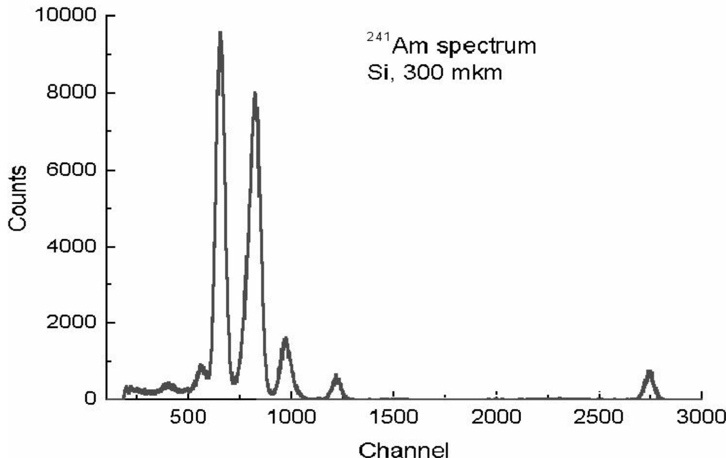
Measurement of radiation of isotope source  $^{241}\text{Am}$  using uncooled detector.
